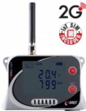
IoT Wireless Datalogger kit with built-in GSM modem and Flat Rate SIM Card allows the instant connection to the COMET Cloud. IoT Datalogger is designed to record temperature, humidity, atmospheric pressure and CO2 from built-in sensors. In case of exceeded set limits e-mail is sent from the [COMET Cloud](#).
