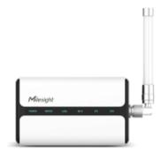
After installation, it immediately begins receiving and sending data messages to and from the LoRaWAN® network via its antenna. This third-party product is supplied with all the original accessories required for power supply and installation.
