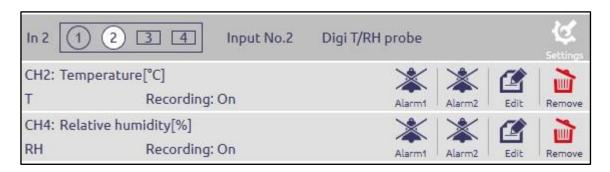
In the line of each measured variable (ie. channel), you can change its other settings (eg. Alarm limits, alarms indication, the channel recording, etc.). For these settings, use *Alarm1*, *Alarm 2* and *Edit* icon.
