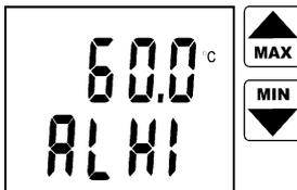
Reading ALHI indicates adjusted upper limit. Set the desired value in the same way as in above lower limit. If needed it is possible to get back to lower limit setting of the same alarm by pressing DISPLAY key. Press ENTER key to confirm new upper limit.
