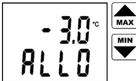
Reading ALLO indicates adjusted lower alarm limit. Set the desired value by means of the arrow keys. Press and hold the arrow key UP to make value increase fast. Press and hold the arrow key DOWN to make value decrease fast. Release the arrow key and press ENTER to confirm new limit.
