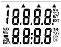
Connect the external probe to the connector before switching ON the instrument. Switch ON the instrument by pressing ON/OFF key. After switching ON the instrument all symbols on the LCD are displayed. If the ON/OFF key is being held pressed, all LCD symbols are displayed till the key is released.
