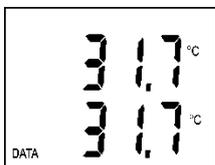
Press HOLD key in the default mode (displaying of actual measured temperature) to store actual measured value to internal memory (indicated by short beep). Anytime it is possible to display stored value from MENU (see below). Each pressing of the HOLD key in the default mode causes value stored in HOLD memory is replaced with actual temperature.
