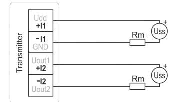
Loop resistance value Rc = Rm + resistance of wires shall fulfill the condition  $Rc[\Omega] < 40 \times Uss[V] - 360$ .
