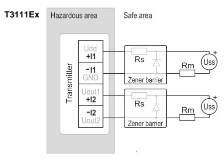
Loop resistance value Rc = Rm + Rs + resistance of wiresshall fulfill the condition  $Rc[\Omega] < 40 \times Uss[V] - 360$ .
