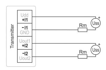
Loop resistance value Rc = Rm + resistance of wires shall fulfill the condition  $Rc[\Omega] < 40 \times Uss[V] - 360$ .
